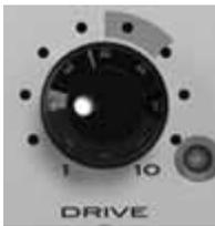
This control allows you to adjust the input signal to optimum levels required for Big Bottom to work effectively. To find the optimum level, turn the control clockwise until the green LED at the right of the Drive control pulses on the bass peaks. Longer and brighter pulsation means a longer bass sustain is being created. You will find a range of settings that yields very musical and powerful bass.
