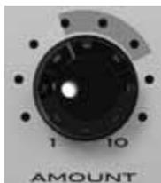
This control varies the amount of enhancement mixed back into the original signal, from the sidechain. Maximum effect is achieved when the control is set fully clockwise.
