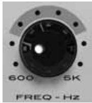
The Aural Exciter Frequency control adjusts the corner frequency of the high pass filter, thus setting the range of frequencies being enhanced by the Aural Exciter. The range of the corner frequency is 600Hz (fully counter clockwise) and 5kHz (fully clockwise). The 12 o'clock setting is approximately 3kHz. As the tune control is adjusted clockwise, less and less mid-frequency enhancement will take place.
