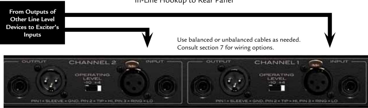
Select the correct OPERATING LEVEL to match your interconnecting equipment. Both the outputs and inputs are switched simultaneously.
